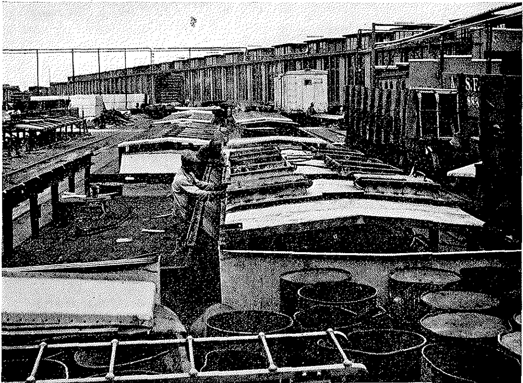
Workmen at Topeka shops repairing doors in roofs of grain or cement hopper cars. A sizeable program is under way to modernize and otherwise improve various classes of Santa Fe freight equipment.
