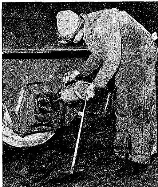
Bill Soffray demonstrating correct way to oil a Journal box.
