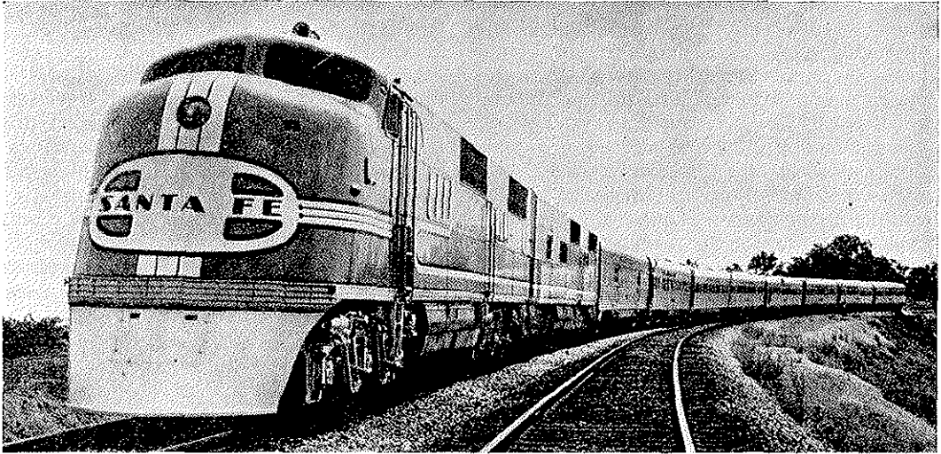
Diesel-electric, 4000 horsepower, two unit locomotive which hauls the Super Chief between Chicago and Los Angeles, 2,227 miles.
