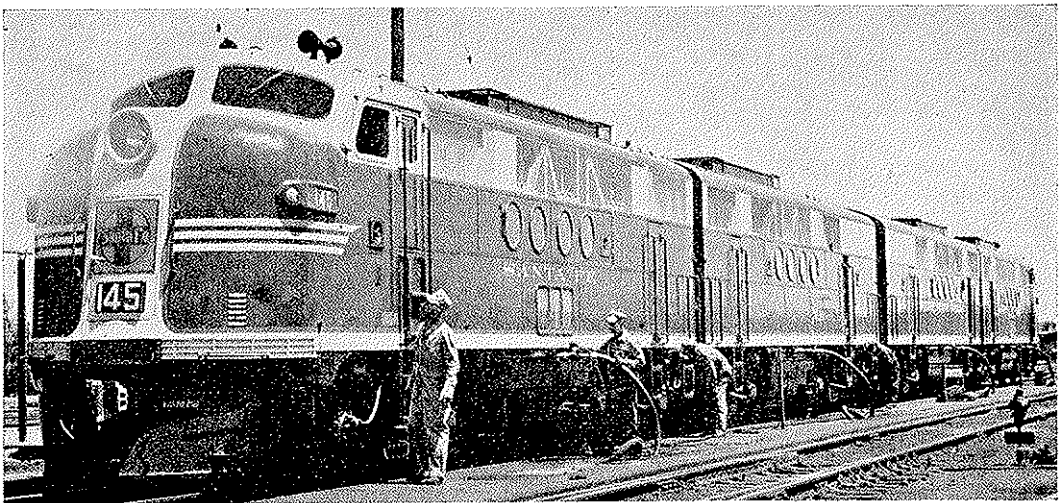
Crew servicing a Diesel freight locomotive at Winslow, Ariz. Photo shows the fuel man, inspector and brake shoe man, and at front of engine John Galvin, dispatching foreman.
