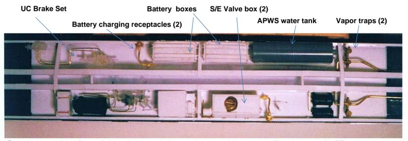
Cut away the flat side channel & replace with true 3D channel: (Evergreen .100") Cut out the original floor from nearly bolster to bolster & replace with a new floor. New floor made from Evergreen sheet flush with the bottom of the old floor depth.
