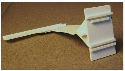
I use a homemade gage to check the car height:
