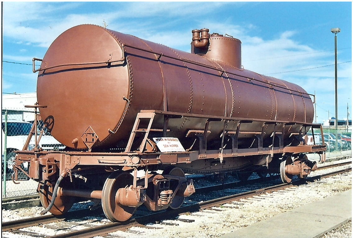
Figure 16. ATSF 100221, B end, right side, fully primed
