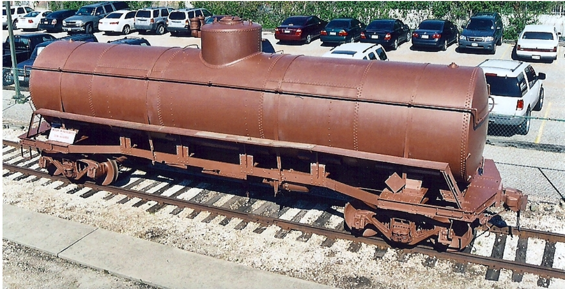
Figure 17. ATSF 100221 top and right side fully primed
