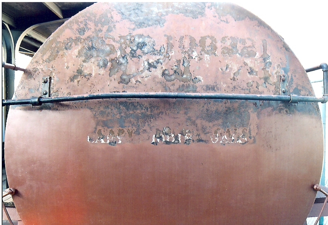
Figure 9. A end showing older and newer car number and capacity stencils.
