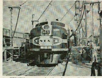
2 TRUCKS are sprayed with a cleaning solution as locomotive leaves sanding platform. An electrical track circuit controls solution sprays automatically.
