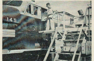
5 CLEANING of cab interior, as well as sterilizing of drinking water containers and miscellaneous servicing tasks is handled at this elevated platform.
